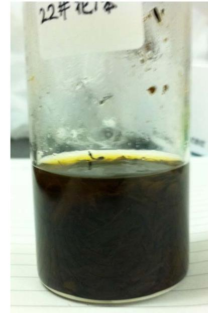
Organic compounds were decomposed by the hydrothermal operation. Most of solid components were decomposed to light-weight compounds, which were dissolved to water phase. Cs is also transferred to water phase.
