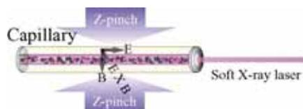
Fig. 1 Capillary discharge pumping
