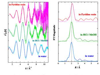
Fig. 1 Nd-L $_{\rm III}$  EXAFS and corresponding fourier transforms for solution samples and resin sample.
