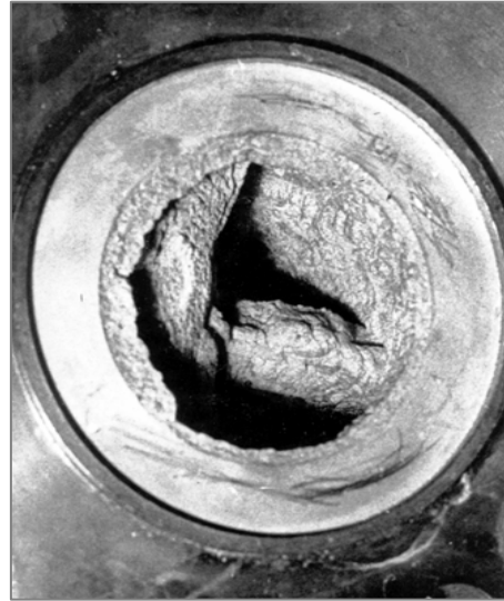
Slag deposits in The vessel
