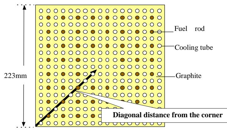
The tentative design of the fuel element has 60 fuel rods and 229 cooling water/steamy tubes.
