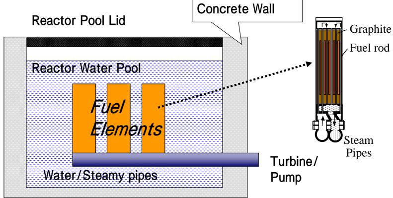
"KAMADO" core consists of fuel elements of graphite blocks, in which UO<sub>2</sub> fuel rods and cooling water pipes are contained. Fuel elements are located in a reactor water pool of atmospheric pressure (1 atm.) and low temperature (< 60  $^{\circ}$ C).
