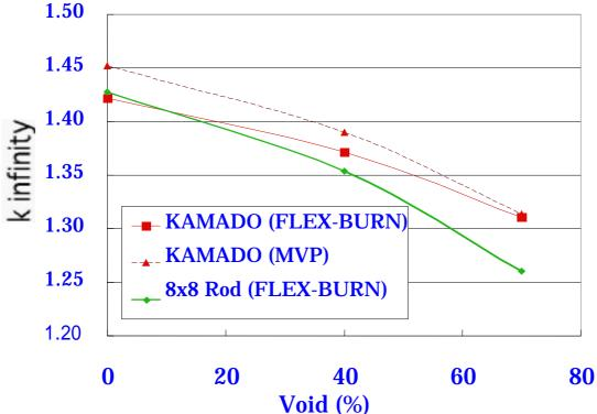
Difference between results of FLUX-BURN and MVP show complexity of resonance shielding on the fuel element consist of  $UO_2$ , graphite and  $H_2O$ .
