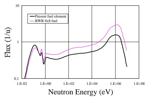
Neutron energy spectrum of the fuel element is a little softer than that of BWR 8x8 type of fuel, because of neutron moderation effect of graphite. RIFPI
