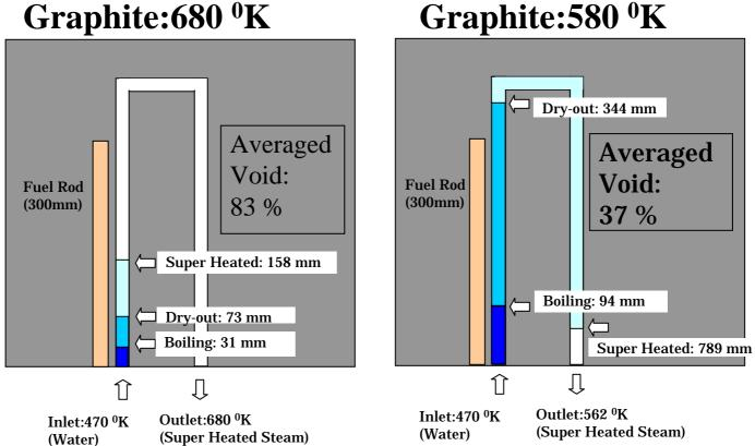
Since cooling water does not contact a fuel rod directly, considerations of **dry-out limitation** and **MCPR** are **not necessary**. Therefore **super-heated steam** is taken out from the fuel element.
