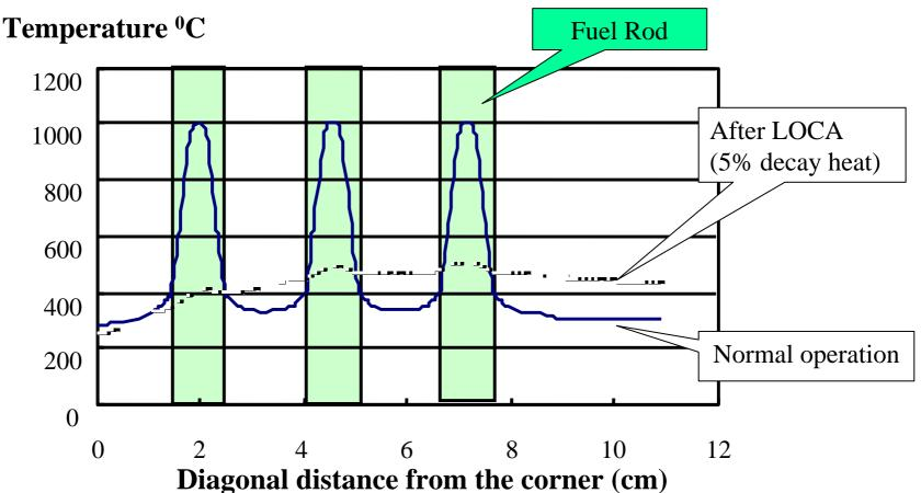
After LOCA (5% decay heat, decay heat at 13 seconds after reactor stop), maximum temperature of graphite is < 500 <sup>o</sup>C without heat removal of cooling water tubes.
