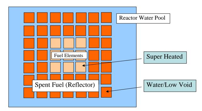
**Spent fuel elements** put on the **reflector region** of the nuclear reactor core, a certain amount of burn-up of nuclear fuel is expectable. If a spent fuel of 60 MWd/kg can be burned more 10 MWd/kg in the reflector region, it will become **effective use** of 17% of **uranium resources**.
