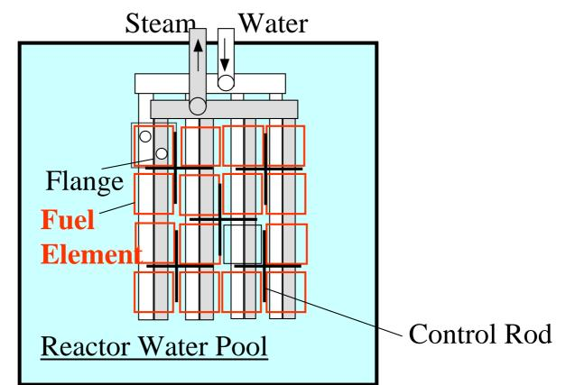
The core consists of two or more **fuel elements**, **control rods**, etc. within the **reactor water pool**.
