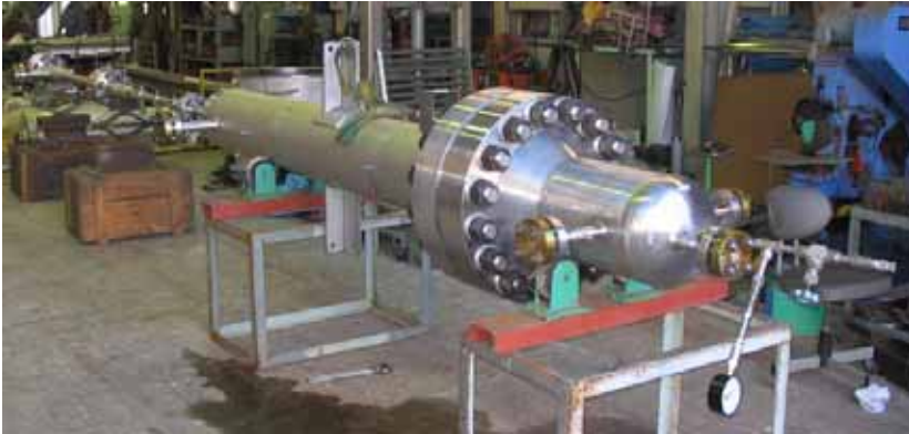
Heater pin bundle, Chimney and Separator
