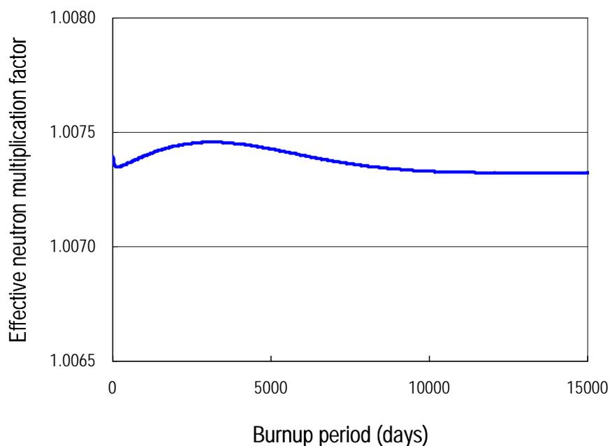
Figure 12 Change in effective neutron multiplication factor with time, obtained by simulation starting from a stationary solution.
