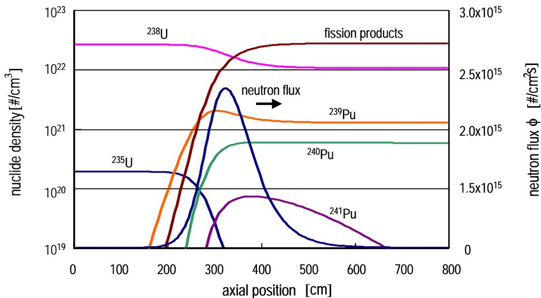
Figure 10 CANDLE burnup in a fast reactor.
