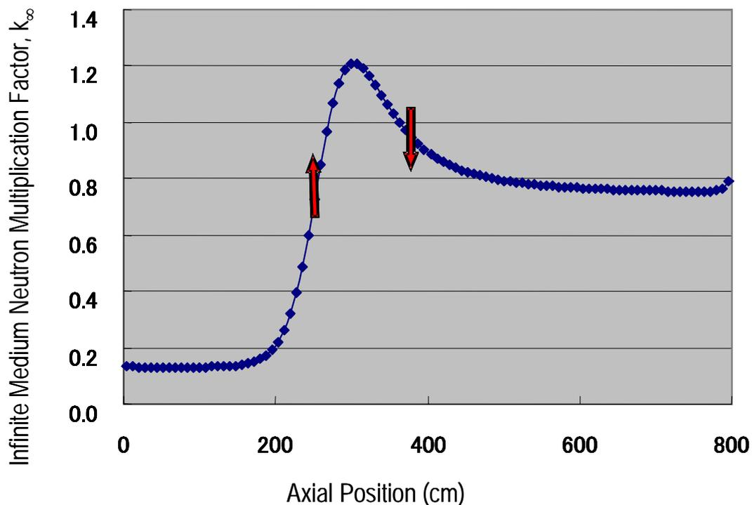
Figure 6 Infinite medium neutron multiplication factor of fuel plotted against the central axis (Z axis). Arrows indicate the directions of change with burnup.
