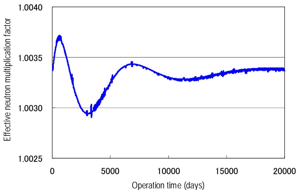
Figure 13 Change in effective neutron multiplication factor with time, obtained by simulation starting from an initial core prepared with easily obtainable materials.
