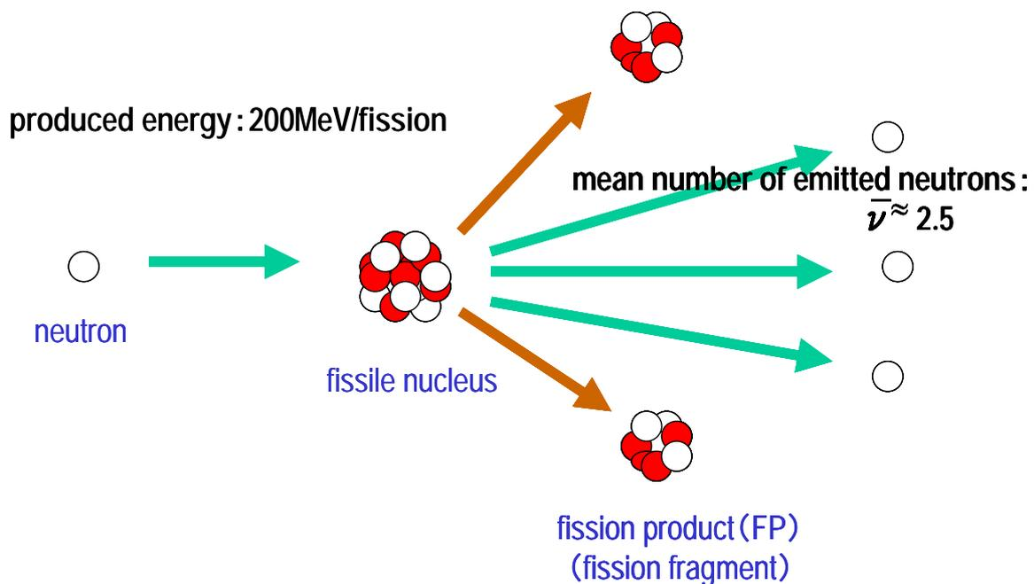
Figure 1 Characteristics of nuclear fission.
