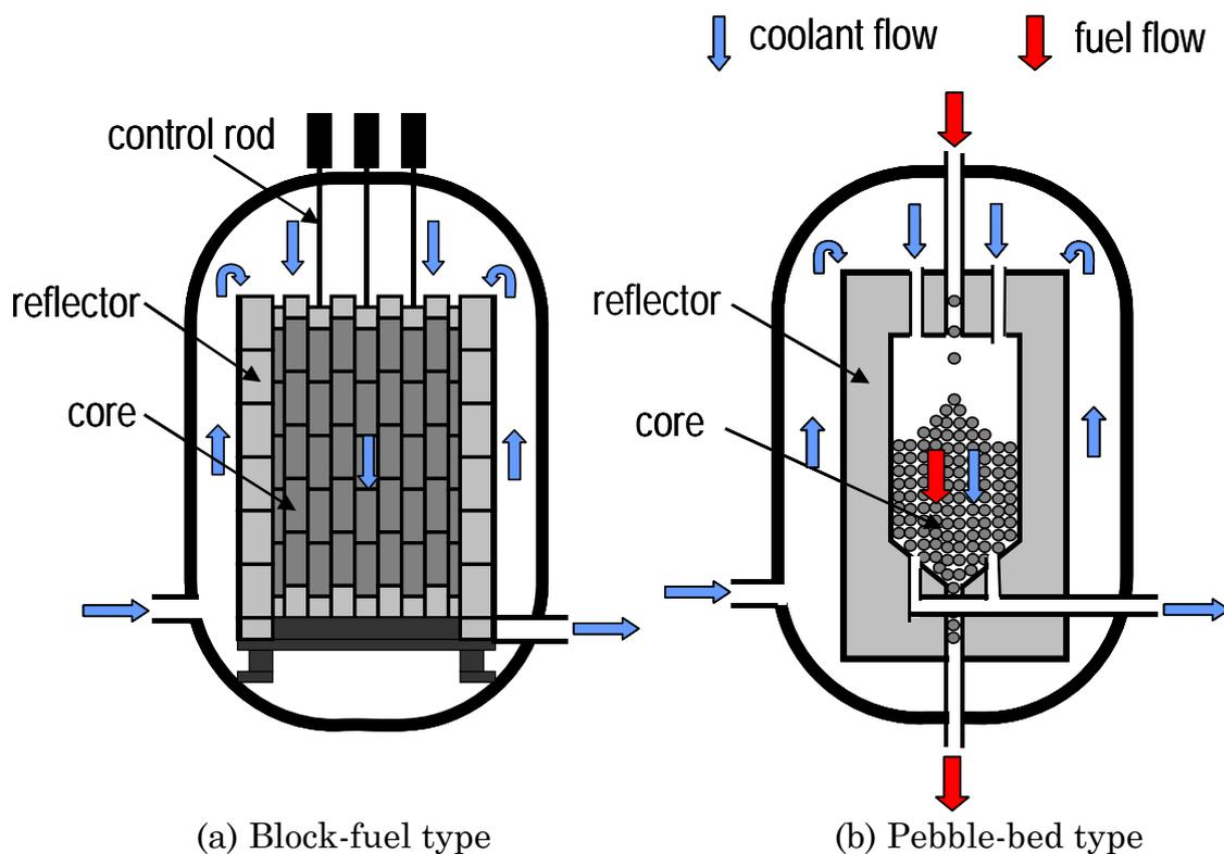
Figure 8 Schematic diagrams of high-temperature gas-cooled reactors.
