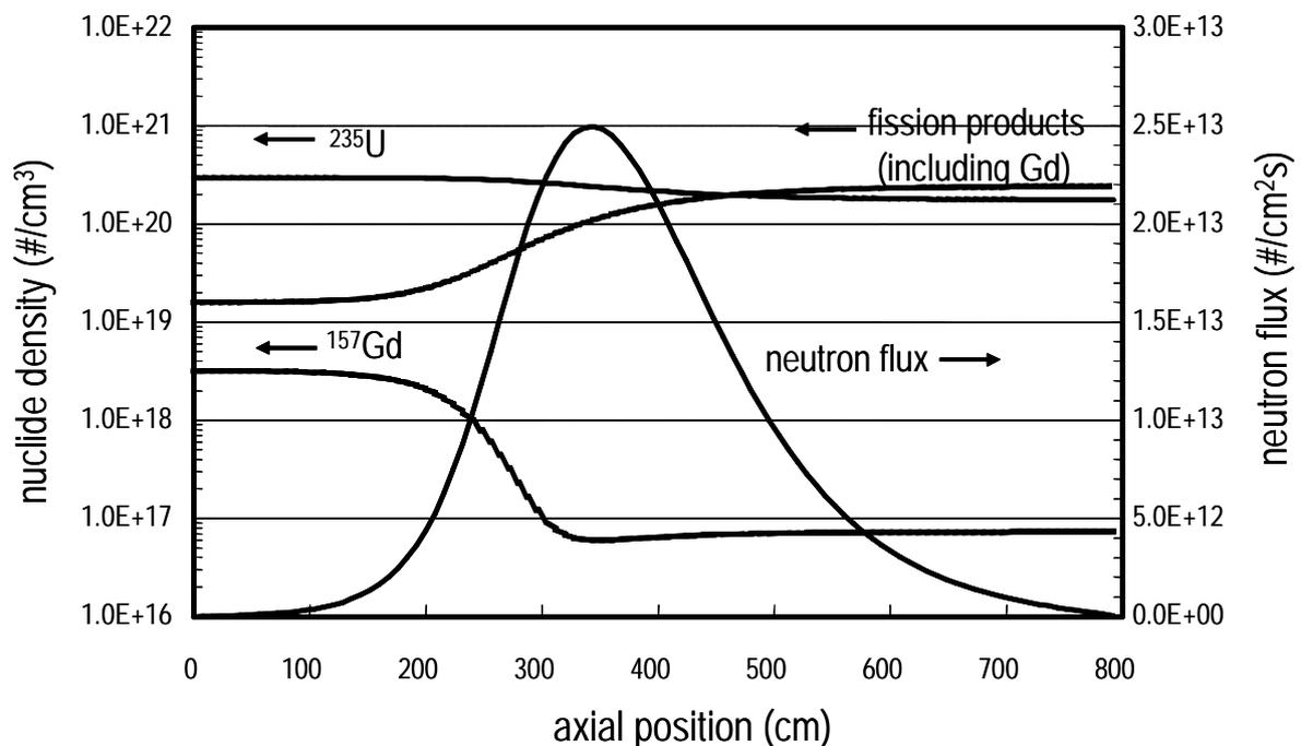
Figure 9 CANDLE burnup in a block-fuel high-temperature gas-cooled reactor.
