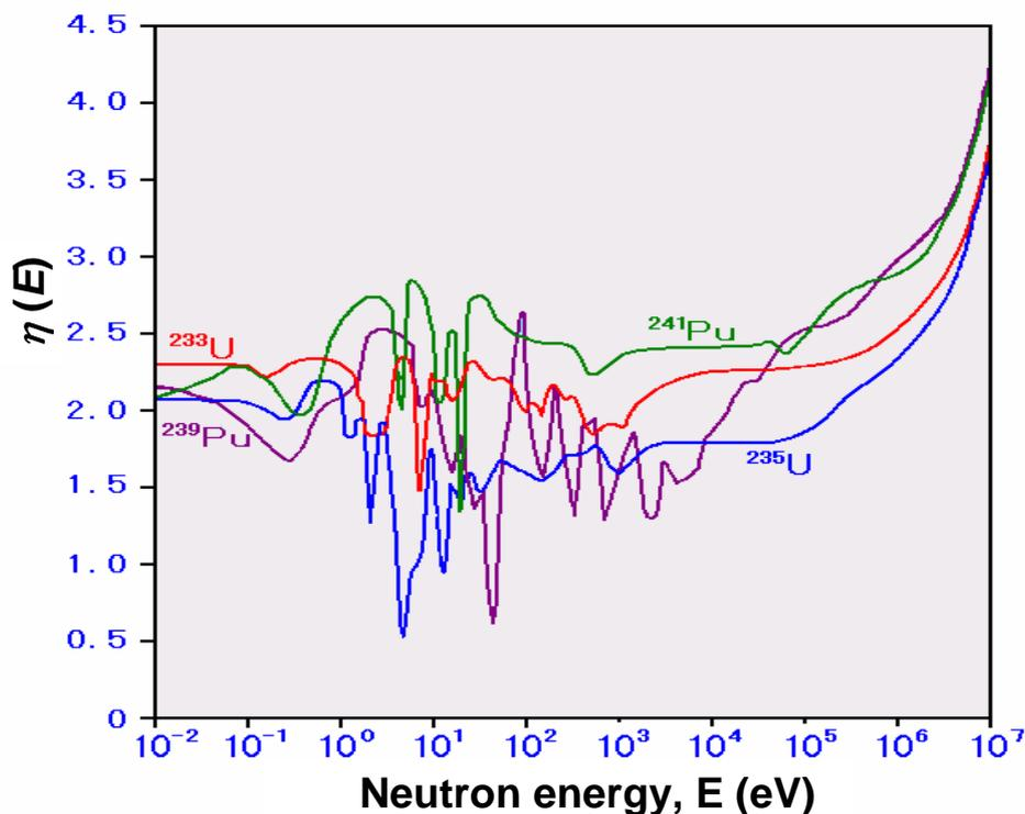
Figure 3 Value of  $\eta$  for typical fissile materials.
