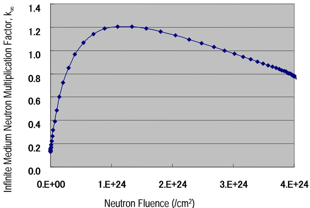
Figure 5 Infinite medium neutron multiplication factor  $k_{\infty}$  of fuel, with neutron fluence plotted on the abscissa.
