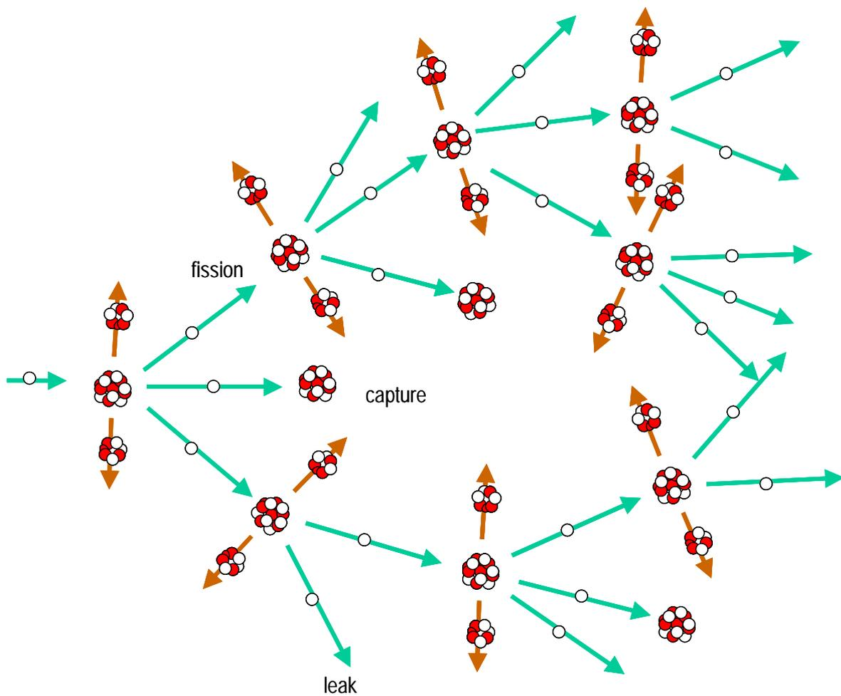
Figure 2 Nuclear fission chain reaction.
