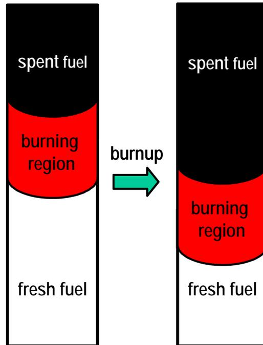
Figure 4 CANDLE burnup strategy. (Note that the moving direction can be the opposite of that illustrated. The core height is illustrated here to be extremely long to make the explanation easy.)
