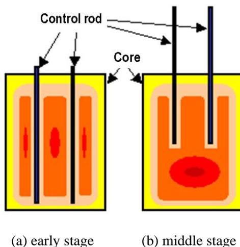
Figure 1. Burn control of conventional reactors (Contour shows power density)
