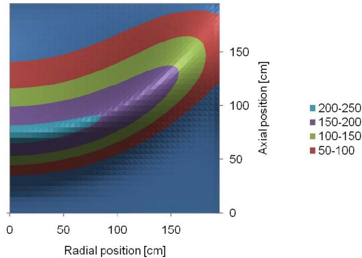
**Figure 4. Steady state power density distribution in a uniform core of CANDLE burnup**
