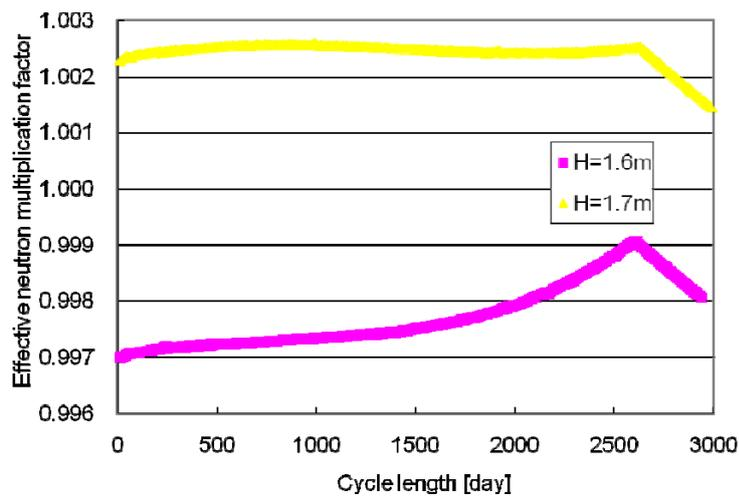
d)  $L=80$  cm**Figure 7. Change of effective neutron multiplication factor for different  $L$  and  $H$**
