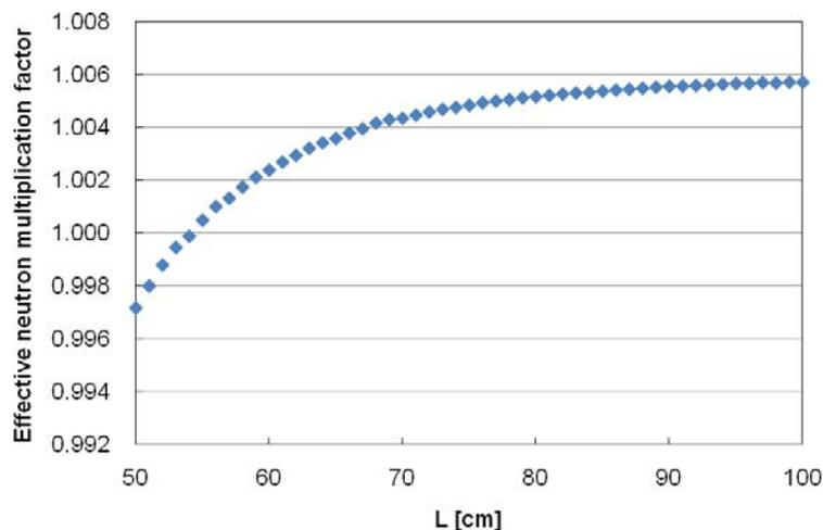
Figure 6. Effective neutron multiplication factor for different  $L$
