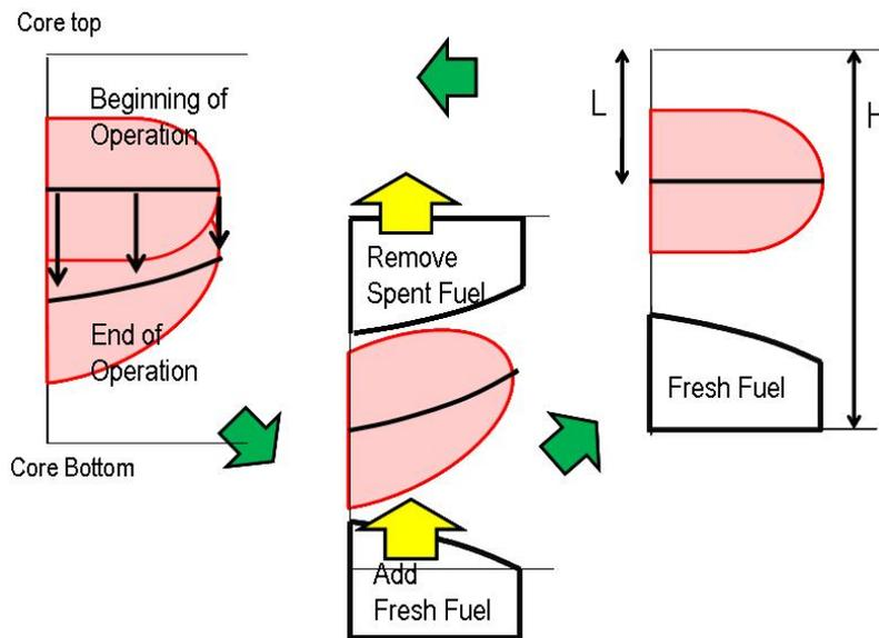
Figure 5. Centroid line of power density distribution for different fuel management stages
