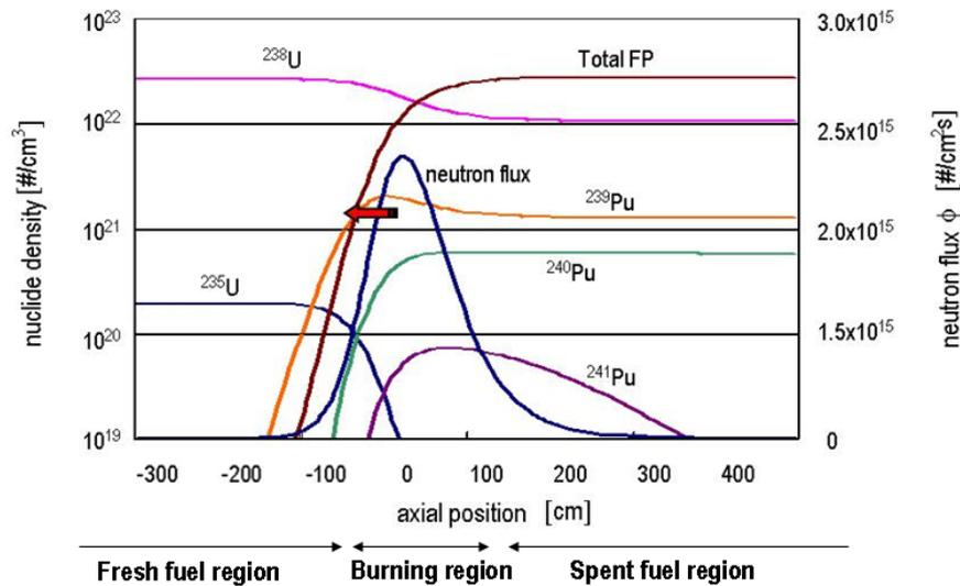
Figure 3. Nuclide densities and neutron flux distributions along core axis
