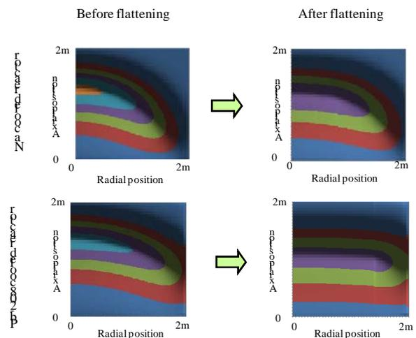
Fig. 4. Two-dimensional power density distributions for Na and Pb-208 cooled reactors before and after flattening
