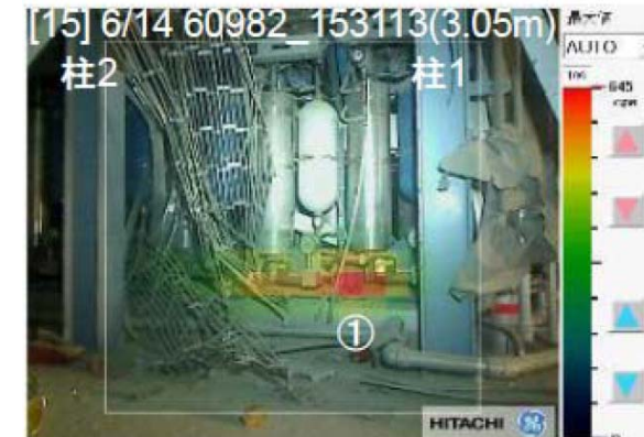
Radiation source survey( \gamma camera) results example (Unit 3 South side HCU)
