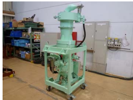
Blaster with cyclone separator
